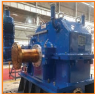
Customer: GE Specification: 63800 kW, 4769 to 1500 RPM Standard: AGMA 6011 J14
