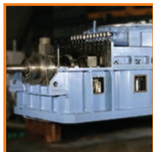
Replacement: Flender Specification: 1600 kW, 990 to 32.8 RPM Application: Vertical Roller Mill Industry: Cement
