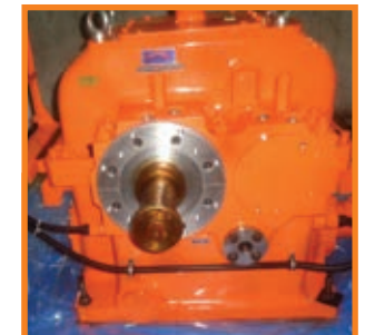
Customer: Elliott Ebara Specification: 785 kW, 5200 to 2980 RPM, API 677 Application: BFW pump
