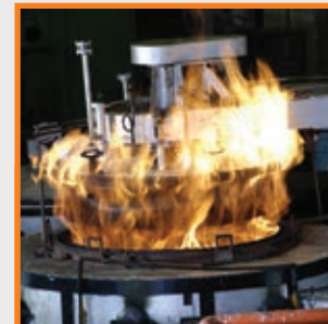
Sophisticated Heat Treatment facility for Carburizing & Nitriding Quenching Tank of 1,00,000 L capacity along with advanced cooling & churning process
