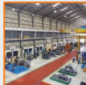
Assembly Bays with a combined handling capacity of 70 tons
