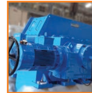
Replacement: Flender Graffenstaden Specification: 36300 kW, 6042 to 1500 RPM Industry: Steel
