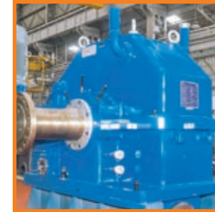
Customer: Siemens Ltd Specification: 56700 kW, 4925 to 1000 RPM Standard: AGMA 6011 J14
