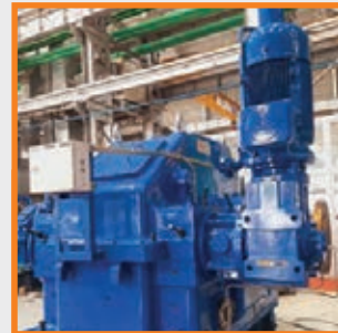
Customer: Skoda Power Specification : 32000 kW, 5468 to 1500 RPM Standard: AGMA 6011 J14
