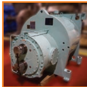
Replacement: MAAG Specification: 600 kW, 1000 to 33.38 RPM Application: HDPE Extruder Industry: Refinery & Petro Chemicals
