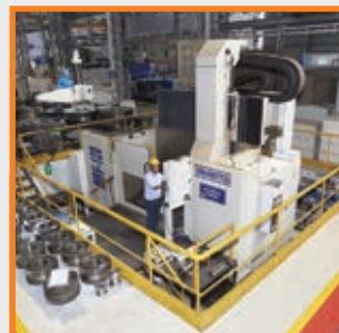
Favretto CNC Vertical Grinding Centre Ø1.2 mtrs.
