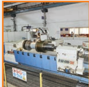
GIORIA Heavy Duty Cylindrical Grinder Travelling Wheel Head Type Ø2X6 mtrs. Length
