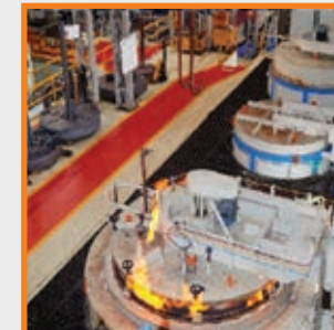
Sophisticated Heat Treatment facility for Carburizing & Nitriding Quenching Tank of 1,00,000 L capacity along with advanced cooling & churning process
