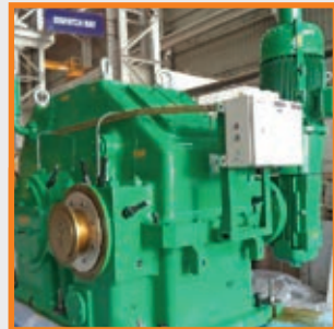
Customer: Man Energy Solutions Specification: 24200 kW, 5595 to 1500 RPM Standard: AGMA 6011 J14
