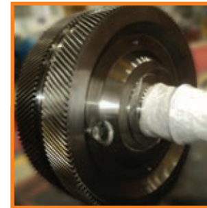
Replacement: Flender Graffenstaden Specification: 43000 kW, 7065 to 1500 RPM Industry: Steel
