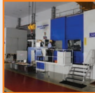
7 Axis CNC Pfauter Gear Profile Grinders with Siemens 840D Control Upto 2.8 meter external grinding, 20 tons table load, 2 meters Internal grinding attachment with Hirth Cutting
