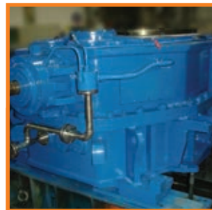
Replacement: David Brown Specification: 260 kW, 970 to 40 RPM Application: Coal Pulverizer Industry: Steel
