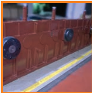
Customer: BHEL Bhopal Specification: 1500 kW, 4000 RPM (1:1 Ratio), 8 Stage, 3 Inputs & 3 Outputs Application: Traction Motor Testing
