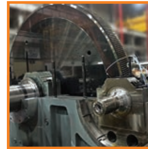
Replacement: BHS Voith Specification: 5000 kW, 1480 to 15581/18094/20775 RPM, API613 Industry: Petro Chemicals
