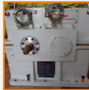
Customer: Voith Specification: 1000 kW, 7000 to 3544 RPM Application: Hydraulic Coupling Testing
