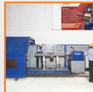
Dynamic Balancing upto 10 tons
