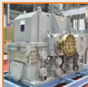
Customer: MHPS Specification: 39000 kW, 7280 to 1800 RPM Application: Load cum Accessory Gearbox
