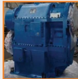
Frame 6 API 613 Replacement to Lenn Mass, USA
