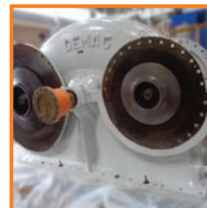
Replacement: Demag Specification: 5300 kW, 5982 to 8376 RPM, API 613 Industry: Steel
