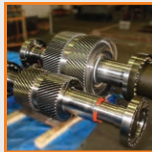
Frame 6 Internals API 613 Replacement to Flender Graffenstaden
