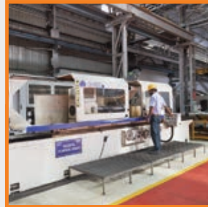
GER Hydraulic Cylindrical Grinder Ø1X3 mtrs. Length
