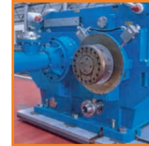
Customer: Man Energy Solutions Specification: 27500 kW, 1500 to 4790 RPM Standard: API 613
