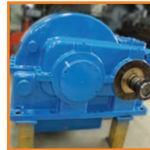
Replacement: MAAG Specification: 15420 kW, 6526 to 3000 RPM Industry: Paper
