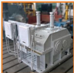
Customer: GTRE Specification: 45 kW, 3000 to 30073 RPM Application: Pump Testing
