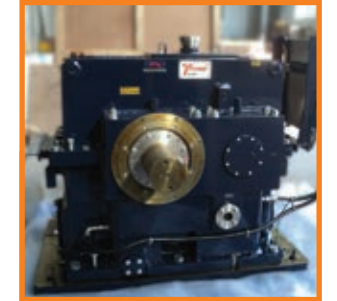
Customer: Atlascopco Specification: 2900 kW, 1480 to 5100 RPM Standard: API613
