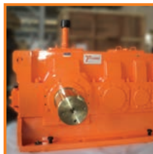
Replacement: Flender Specification: 559 kW, 1500 to 30.55RPM Application: Mill - Cane Crushing Industry: Sugar
