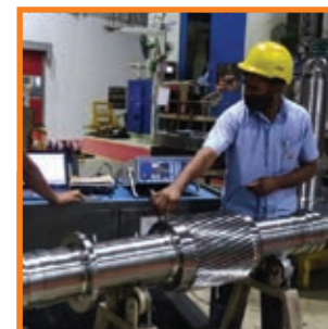
Replacement: MHI Specification: 16330 kW, 8025 to 11787 RPM, API 613, Industry: Steel
