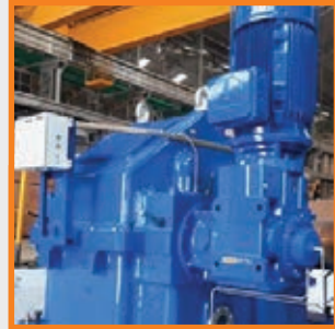
Customer: BHEL Specification: 41000 kW, 5650 to 3000 RPM Standard: API 613
