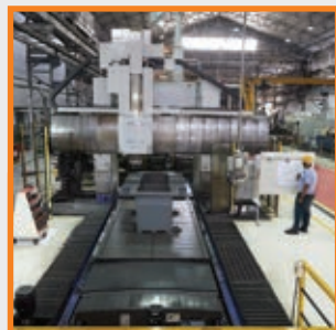
Mitsubishi Double Column Milling Machine with 4 mtrs Traverse & 25 tons capacity
