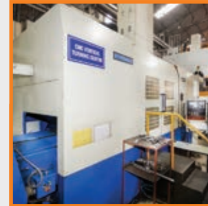
Premier CNC Vertical Turning Centre swing 2.3 mtrs.
