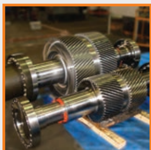
Customer: BHEL Specification: 54000 kW, FRAME 6 Application: Gas Turbine
