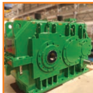
Replacement: Guangzhou Specification: 450 kW, 1000 to 38.4 RPM Application: Extruder Industry: Rubber
