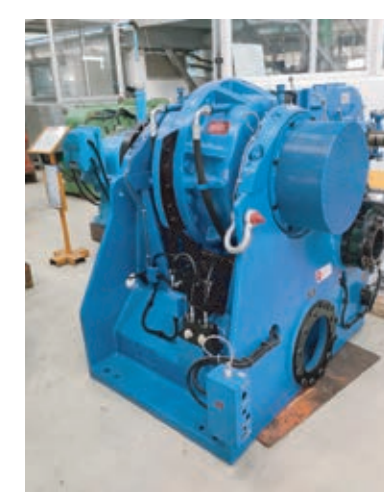
Partial Load Testing upto 1.2 MW
