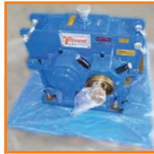
Replacement: Ebara Specification: 162 kW, 2965 to 12981 RPM, AGMA Industry: Refinery
