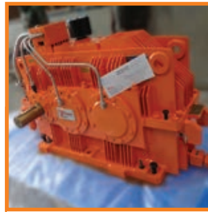
Replacement: Nippon Specification: 395 kW, 1480 to 178 RPM, AGMA Industry: Chemicals and Fertilizers
