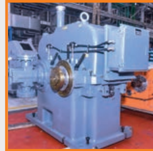
Customer: Triveni Turbines Specification: 24990 kW, 6150 to 1800 RPM Standard: AGMA 6011 J14
