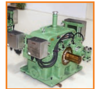
Customer: Sulzer Specification: 1520 kW, 3735 to 1560 RPM, API 613 Application: Boiler Feed Pump
