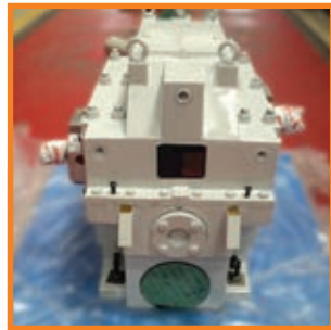
Replacement: Pomini Farrel Specification: 237 kW, 4750 to 754 RPM, AGMA Industry: Chemicals and Fertilizers
