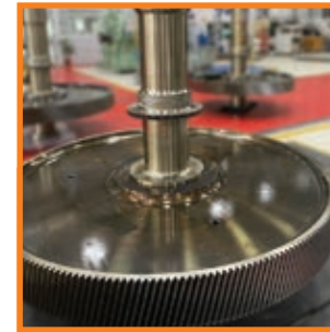
Replacement: Siemens Specification: 4650 kW, 9138 to 10751 RPM, API 613, Industry: Steel
