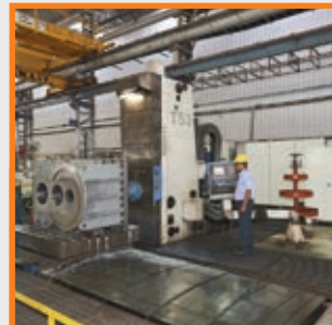
Juaristi Horizontal Boring Machine ATC with 60 tools, 4X2 Mtrs. Traverse
